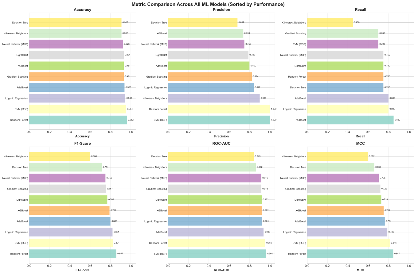
FIG. 6. Performance comparison of ten machine learning models across six evaluation metrics: Accuracy, Precision, Recall, F1-Score, ROC-AUC, and MCC. The models are sorted by performance for each metric (ascending), highlighting Random Forest as the top performer in Accuracy, F1-Score, and MCC, while SVM (RBF) achieves the highest Precision and ROC-AUC scores.
